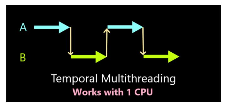
There is still another problem though. TMT is usually implemented based on clock signal. By creating an interrupt handler for clock interrupts, we can manage to change the states of two programs somehow. A program itself never knows it has been suspended.
